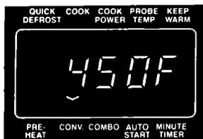
When the oven temperature reaches 450°F, the oven beeps twice and the PREHEAT Indicator Light goes off. "450F" will stay on the Display and the oven will hold that temperature up to 30 minutes, or until the food has been placed in the oven and START has been touched. **NOTE: The oven will automatically shut off and the Display will show the time of day if food has not been placed in the oven within 30 minutes.**
